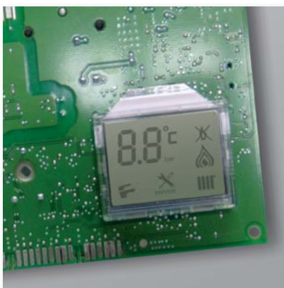
HONEYWELL electronic PCB with microprocessor
